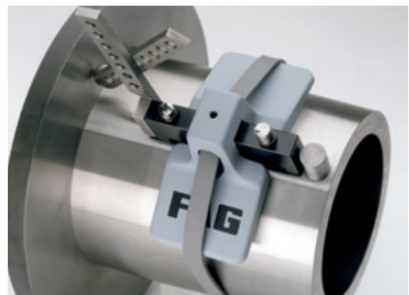
Figure 5: Taper measuring instrument attached to the side of a journal
