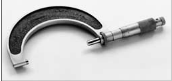
2: External micrometer for measuring shaft diameters
