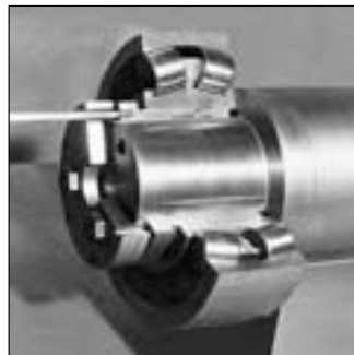
99: Dismounting a withdrawal sleeve mounted spherical roller bearing by the hydraulic method.
