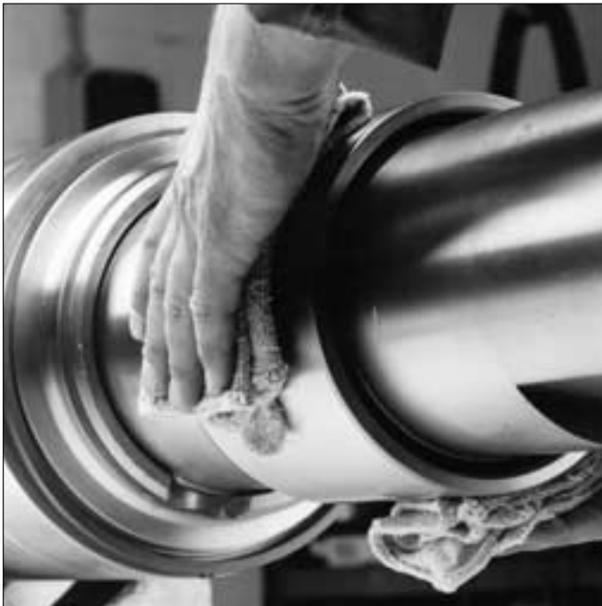
41: Heated bearing parts are rapidly pushed on the shaft and positioned squarely against the shoulder. This is facilitated by a slight twisting motion.
