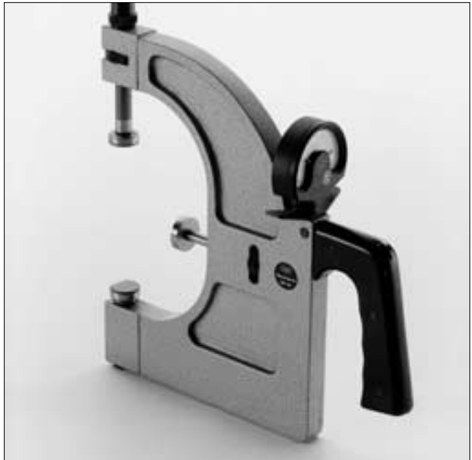
3: A snap gauge ensures safe positioning and perfect measurement of cylindrical seats. The diameter for setting the gauge is marked on the master ring.
