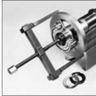
81: Dismounting of a barrel roller bearing with an extractor
